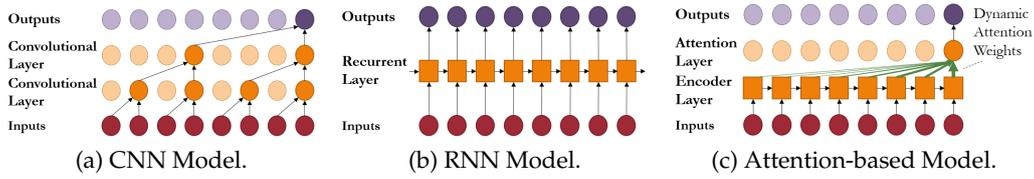
Figure 1: Incorporating temporal information using different encoder architectures.
